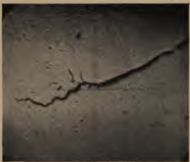
NO. 53. SLAG CRACK NEAR EDGE IN SOLID METAL.
